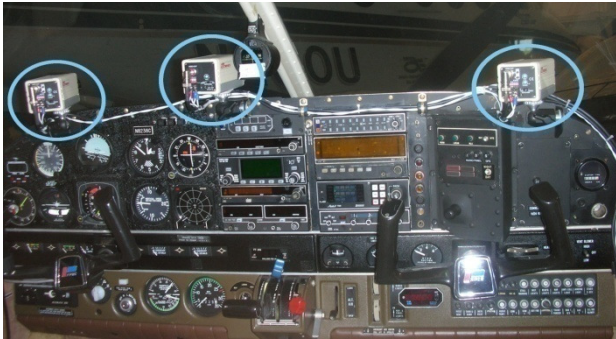
Figure 3. Three Camera Installation
